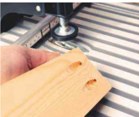
The resulting pockets are clean and uniform
